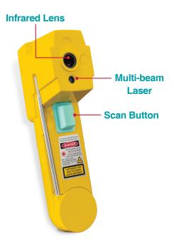
Distance:Spot (FOV) = 8:1 (FOV = Field of View) Emissivity = 0.1 to 1, Step 0.01
